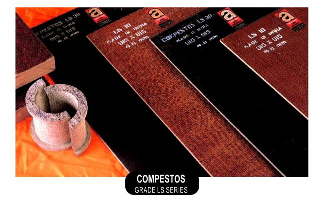
Asbestos laminated sheets are moulded from Asbestos Cloth with thermosetting resins and are specially developed for engineering applications. The high content of Asbestos, superior grade of binder and special press-curing technique impart high degree of mechanical strength. These materials are hard wearing, heat resistant and unaffected by a wide range of chemicals and solvents.
