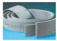
is a flexible moulded, non-metallic friction material, light grey or brown in color and having a random fibre asbestos base. It is available in roll and strip form and is suitable for use under dry operating conditions only (i.e. it is not suitable for use in oil).
