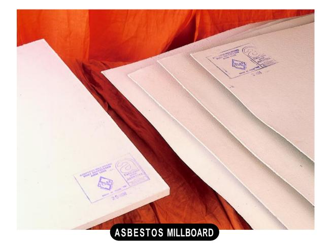
This is a versatile, thermal insulation and heat-resistant material produced in sheet form using good quality asbestos fibres, incombustible fillers and vegetable binders. It does not suffer loss of strength upto 485°C. When suitably supported the board can be used satisfactorily at extreme temperatures upto approx. 1400°C.
